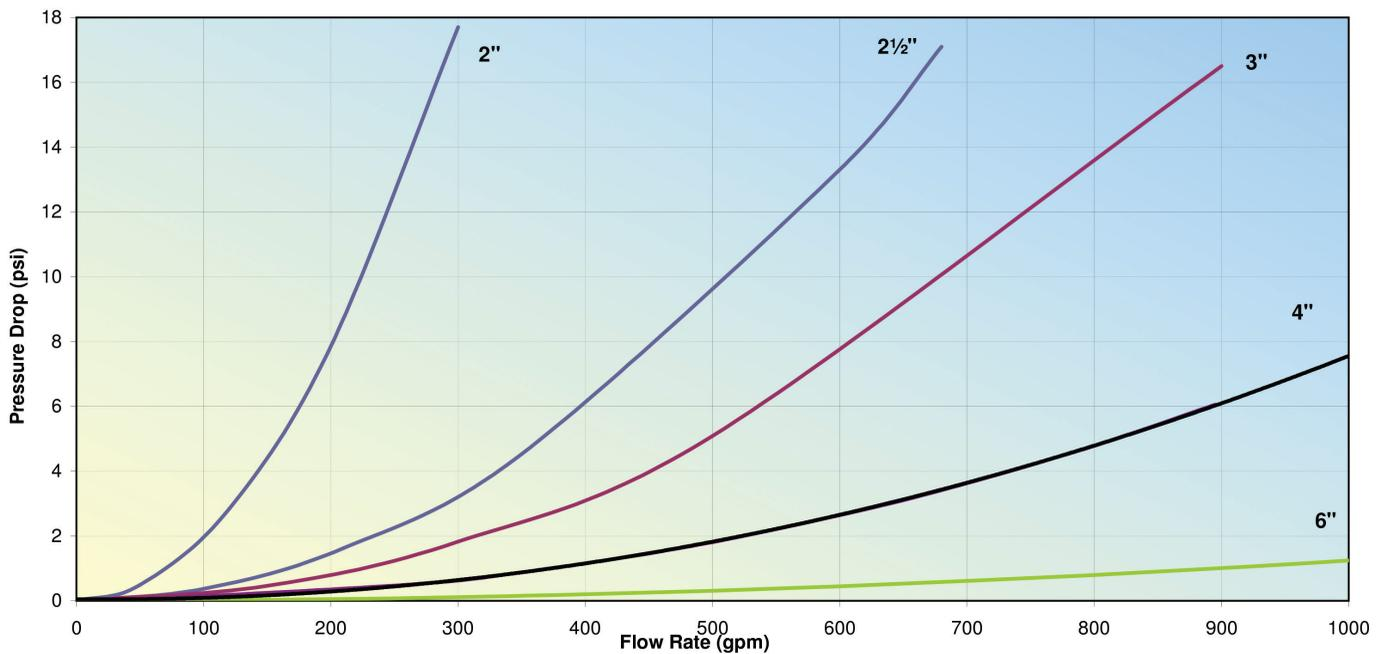
Test Fluid: LNG    Temperature: -256 °F    Density: 27.2 lbs/ft<sup>3</sup>    Viscosity: 0.11 cps
